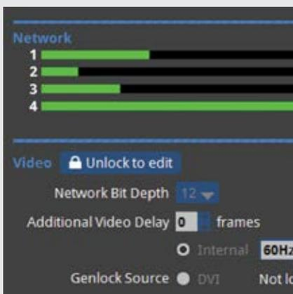
Load bars give visual indication of remaining network capacity at chosen bit depth and frame rate.
