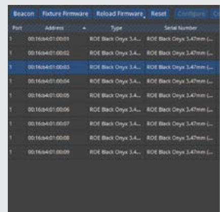
Detected fixtures are available in a tabular view, providing a quick way to perform tasks such as firmware reload.
